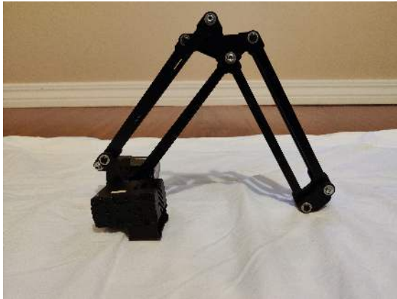
(a) Link Assembly: Side View
